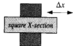
Prismatic (P) joint—1 DOF
